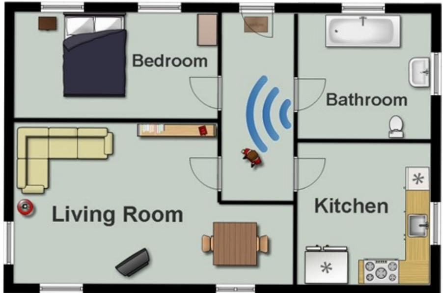
You should install the **SeN-Cit** unit in the area of the home where you would expect regular movement, typically on the landing or in a hallway. The **SeN-Cit+** door sensor can be mounted up to 30m from the main **SeN-Cit+** unit and should be fixed to the main door of the home.
